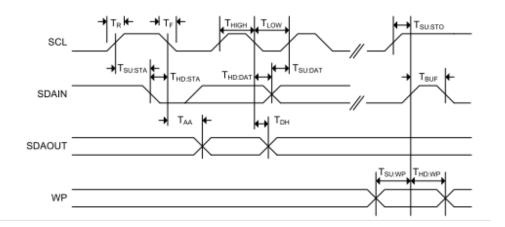
Figure 12. Write Cycle Timing
